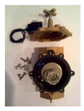
**2.** Remove spring and diaphragm assembly from valve body
