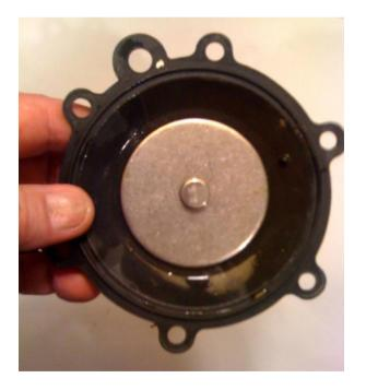
Photo below shows bottom side of diaphragm assembly which includes cone shaped seat which descends down into brass seat of valve body when valve is in closed position
