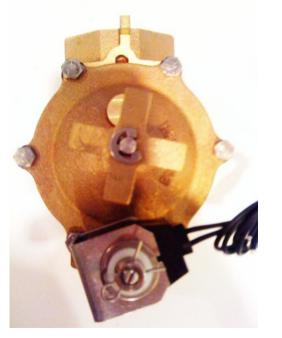
**2.** Lift coil and U-frame off of the solenoid post.
