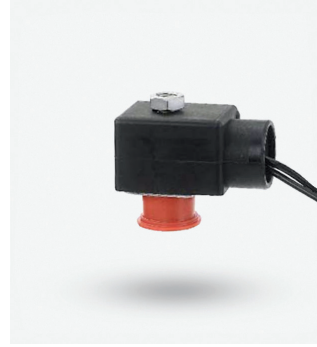
16275 110 VAC In Rush Current: 95 mA (10.5 VA) Holding Current: 65 mA (7.2 VA) Compatible with: SPV, 450, 950
